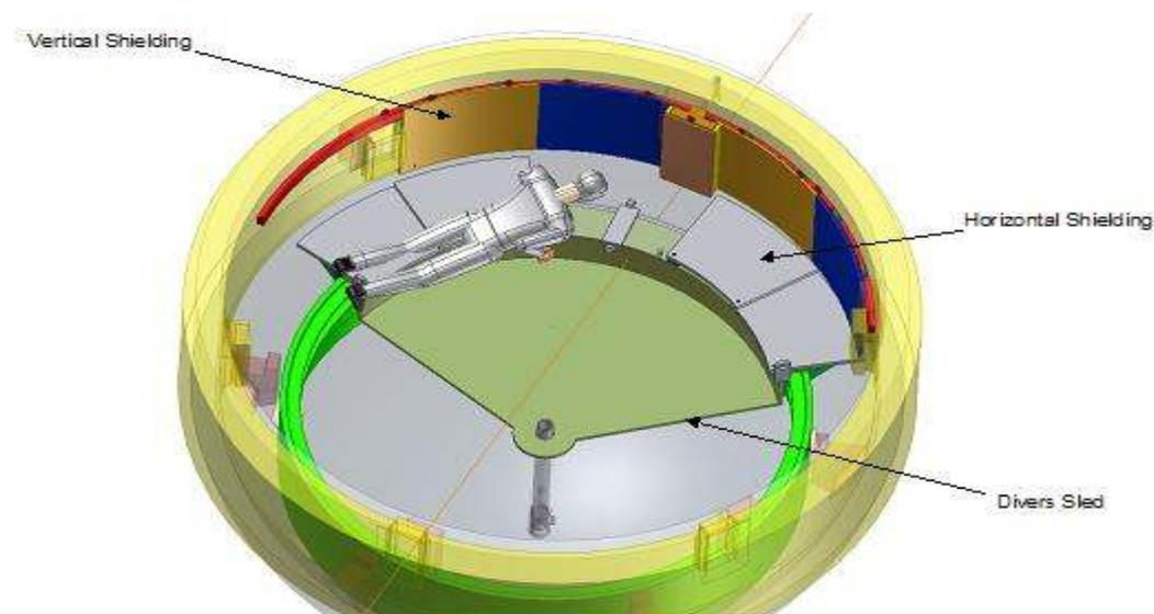
[Picture 11] Diver Sled and the Establishment Status of Shielding
