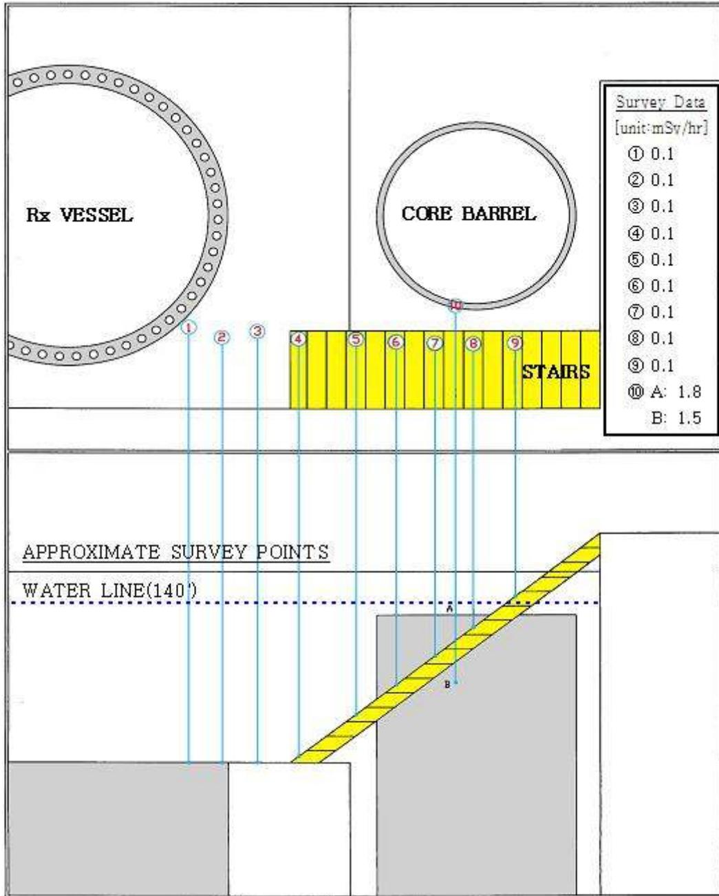
[Picture 8] Reactor Cavity Survey Map
