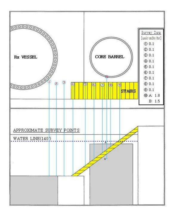
[Picture 8)] Reactor Cavity Survey Map
