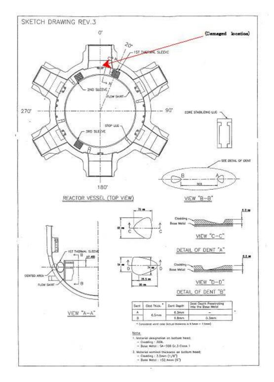
[Picture 2)] The location of internal cladding defected at Rx Vessel
