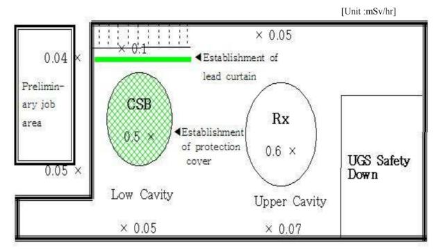
[Picture 9)] Radiation dose rate of Rx cavity area
