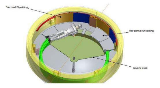
[Picture 11] Diver Sled and the Establishment Status of Shielding
