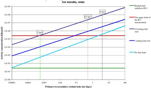
Activity detected by RY-monitor as a function of leak size hot standby -state
