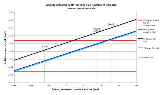
Figure 8. The relationship between leak size and activity detected by RY-monitor, power operation.
