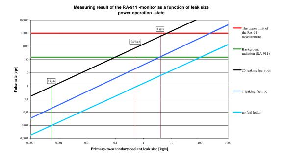
**Figure 9.** The relationship between leak size and measurement of the RA-911-monitor, power operation. Figures 10-11 are graphs of hot standby -cases:
