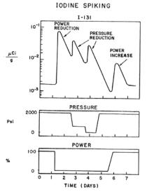
Figure 2. Schematic representation of iodine spiking [2].
