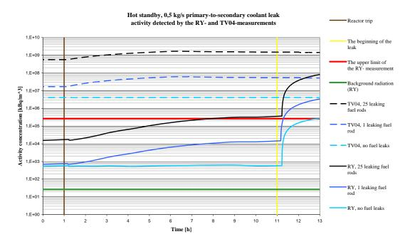
Figure 5. 0,5 kg/s p-to-s leakage in hot standby, RY- and TV04-monitors
