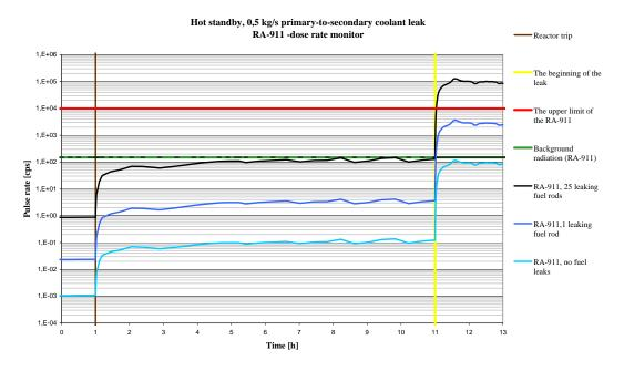
Figure 7. 0,5 kg/s p-to-s leakage in hot standby, RA-911-monitors
