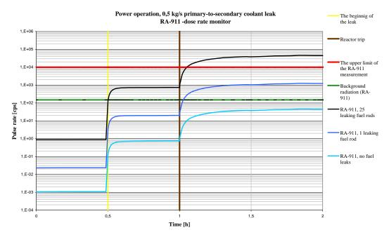
Figure 6. 0,5 kg/s p-to-s leakage in power operation, RA-911-monitors
