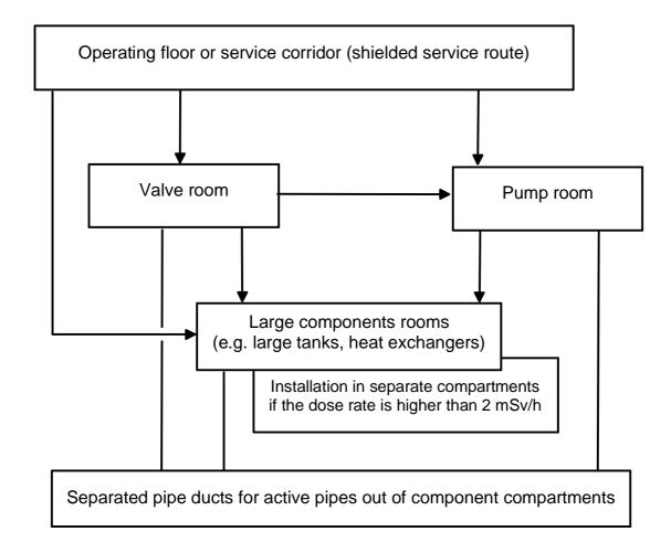
Figure 3: Principle scheme of compartment access
