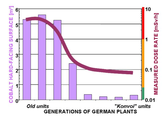
Figure 2. Illustration of the link between cobalt hard-facing and dose rate
