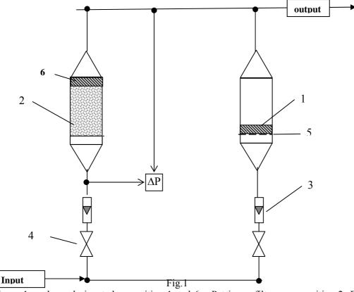
In the figure 1 we have designated as position 1 and 6 – Petrianov filter; as a position 2- BGF; as a position 3 – rotameter; as a position 4 – valve; as a position 5 – the grid; as a  $\Delta P$  - liquid differential manometer;
