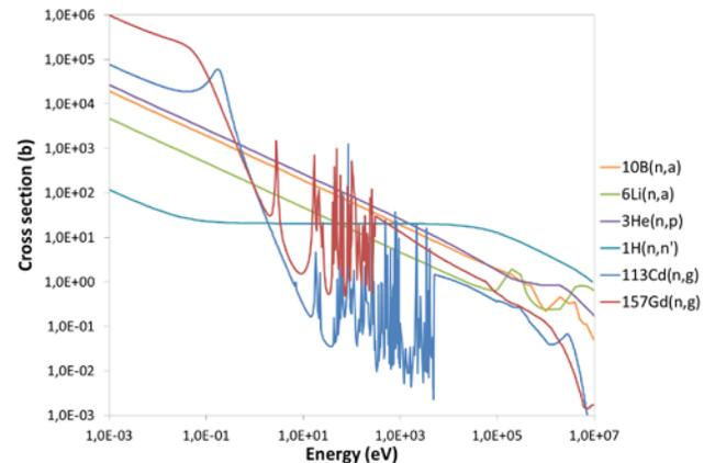
Fig. 1 Cross-sections of different isotopes used for neutron detection.
