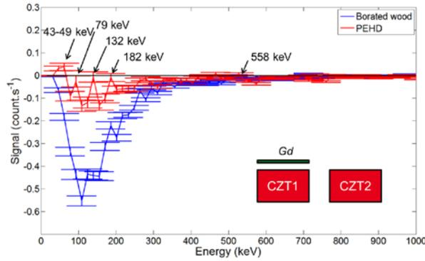
Fig. 7 Subtracted spectra measured without cover on the guard sensor.
