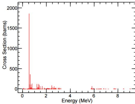
Fig. 2 Prompt gamma-ray emission spectrum of  $^{113}\text{Cd}$  (extracted from IAEA data base [15]).
