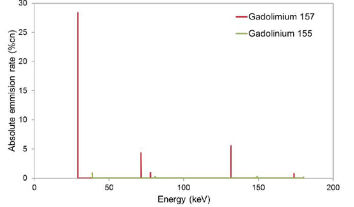
Fig. 4 Internal conversion electron spectrum of  $^{155}\text{Gd}$  and  $^{157}\text{Gd}$  (extracted from IAEA data base [15] and BrIcc conversion coefficient calculator [16]).
