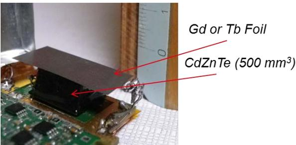
Fig. 5 CdZnTe diode covered by a Tb foil.
