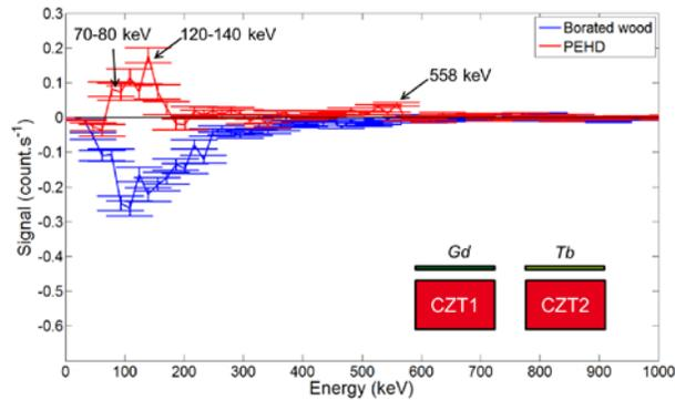
Fig. 8 Subtracted spectra measured with a Terbium cover on the guard sensor.
