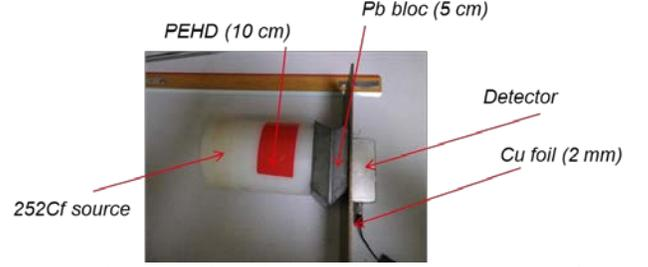
Fig. 5 Experimental configuration maximizing the thermal neutron flux.
