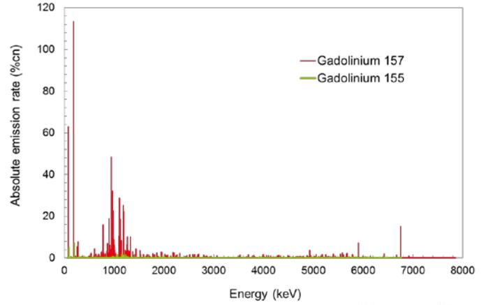
Fig. 3 Prompt gamma-ray emission spectrum of  $^{155}\text{Gd}$  and  $^{157}\text{Gd}$  (extracted from IAEA data base [15]).
