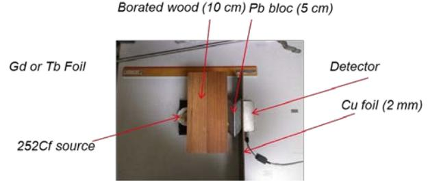
Fig. 6 Experimental configuration minimizing the thermal neutron flux.
