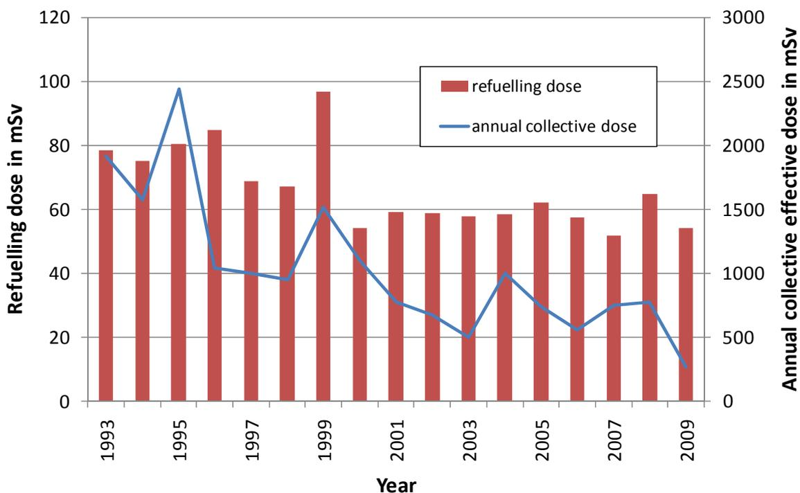
**Fig 8:** The refuelling dose (left scale) and the annual collective effective dose (right scale) in an arbitrarily chosen NPP since 1993
