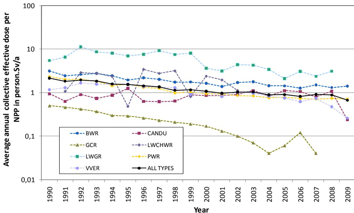
**Fig 1:** The average annual collective effective dose per (operational) NPP of a reactor type in person.Sv/a during the last 2 decades
