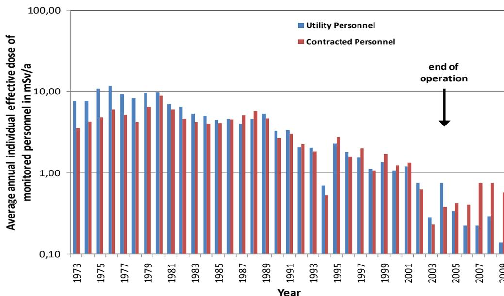
**Fig 6:** The average annual individual effective dose in mSv/a during operation and decommissioning of an arbitrarily chosen German NPP
