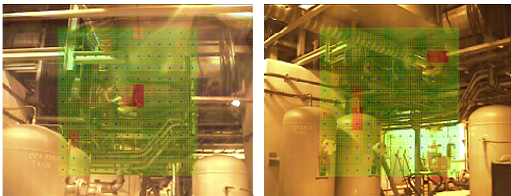
Fig. 4. Gamma scan intensity overlay image taken from two scanning positions (red indicates higher gamma intensity).
