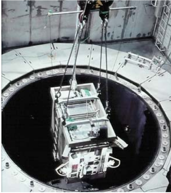
Picture 1: The lead box hanging in the reactor hall crane.
