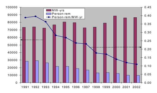
Figure 1: Collective radiation exposure and electricity generated at US nuclear power plants
