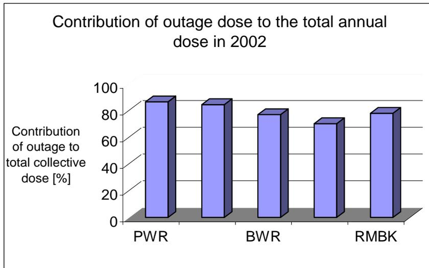
FIG. 4. Average contribution of the outage dose to the total annual dose in 2002 for different types of reactor from in the year 2002.
