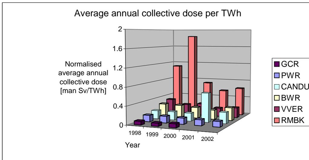
FIG. 3. Normalised average annual collective dose for different types of reactor from the year 1998 to 2002.
