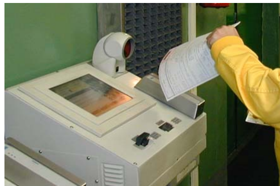
Picture 3: Data station of Electronic Personal Dosimetry System – input to controlled area
