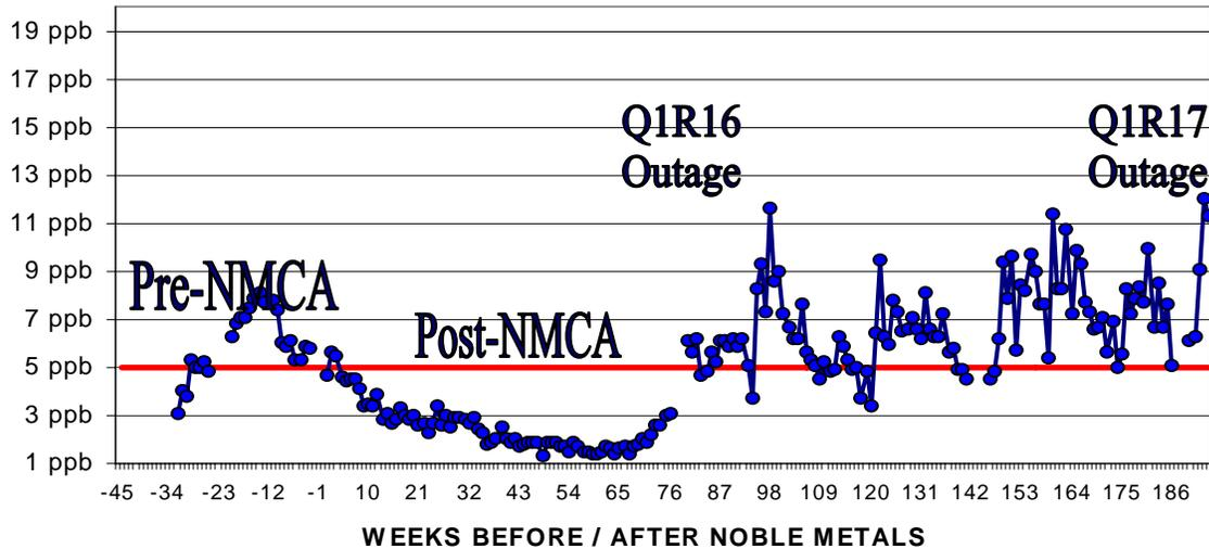
During cycle 17, DZO has been maintained in the 5-10 ppb range. Additionally, hydrogen cycling has been minimized. The soluble and insoluble Co-60 levels have stabilized and even begun to decrease, particularly in the case of the soluble form.
