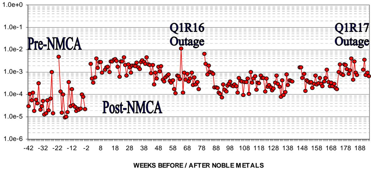
Similarly, soluble Co-60 concentrations were also seen to increase by a factor of two following NMCA application. Currently, soluble Co-60 has begun to steadily decrease as the combination of DZO/hydrogen management and increasing RWCU flow-rate take effect.
