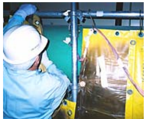
Example of an uncollimated, on-contact measurement.
