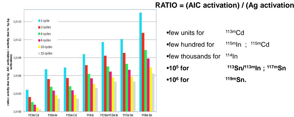
The higher the ratio is, the more selective the indicator is. consequently, a relevant tracer of an AIC control rod leaking can be selected among the following isotopes: <sup>119m</sup>Sn, <sup>117m</sup>Sn and <sup>113</sup>Sn /<sup>113m</sup>In.
