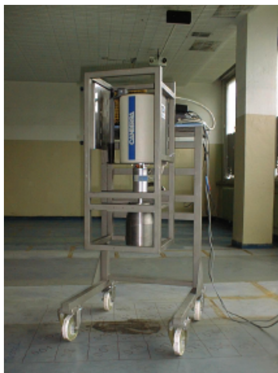
Figure 2: Collimated in situ gamma spectrometer developed in the framework of (5).
