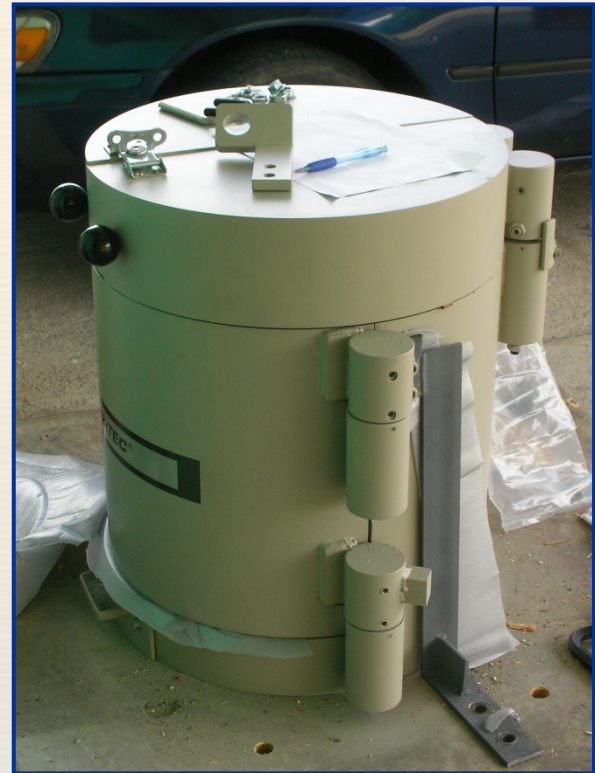
New low-energy gamma spectrometer
