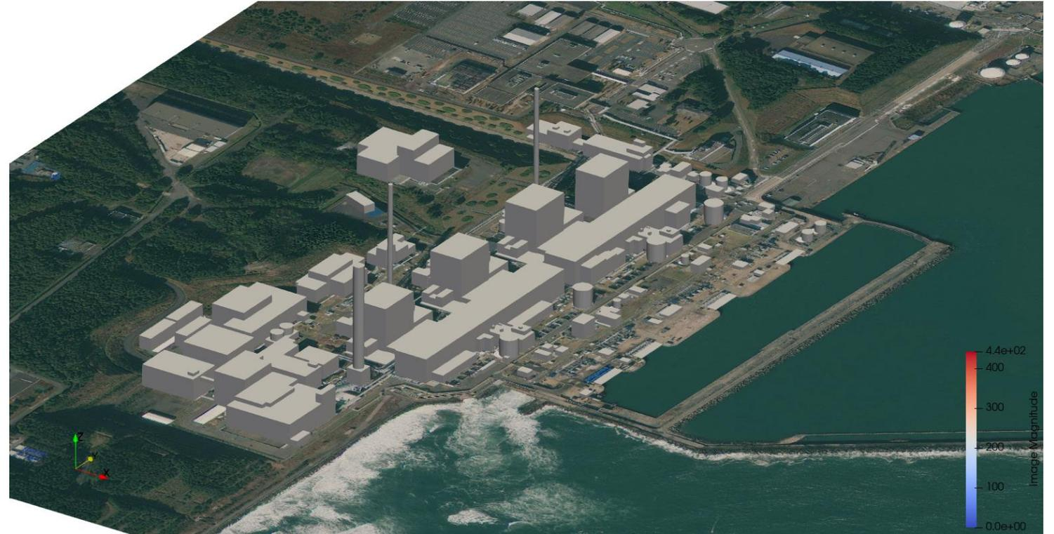
Geometry for the CFD calculation
