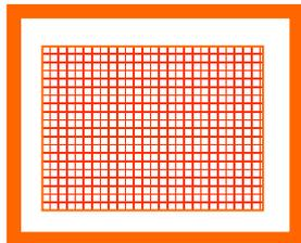
In original design, high density racks are installed in SFP to accommodate spent fuel assemblies **for 20 years**. (1150 fuel assemblies)
