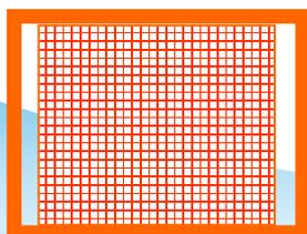
At the stage of operation, SFP is **fully filled** with high density racks **for 25 years** (original 20 years + additional 5 years : final total assemblies are 1450). Increased SFP capacity is about 26% compared with original design.
