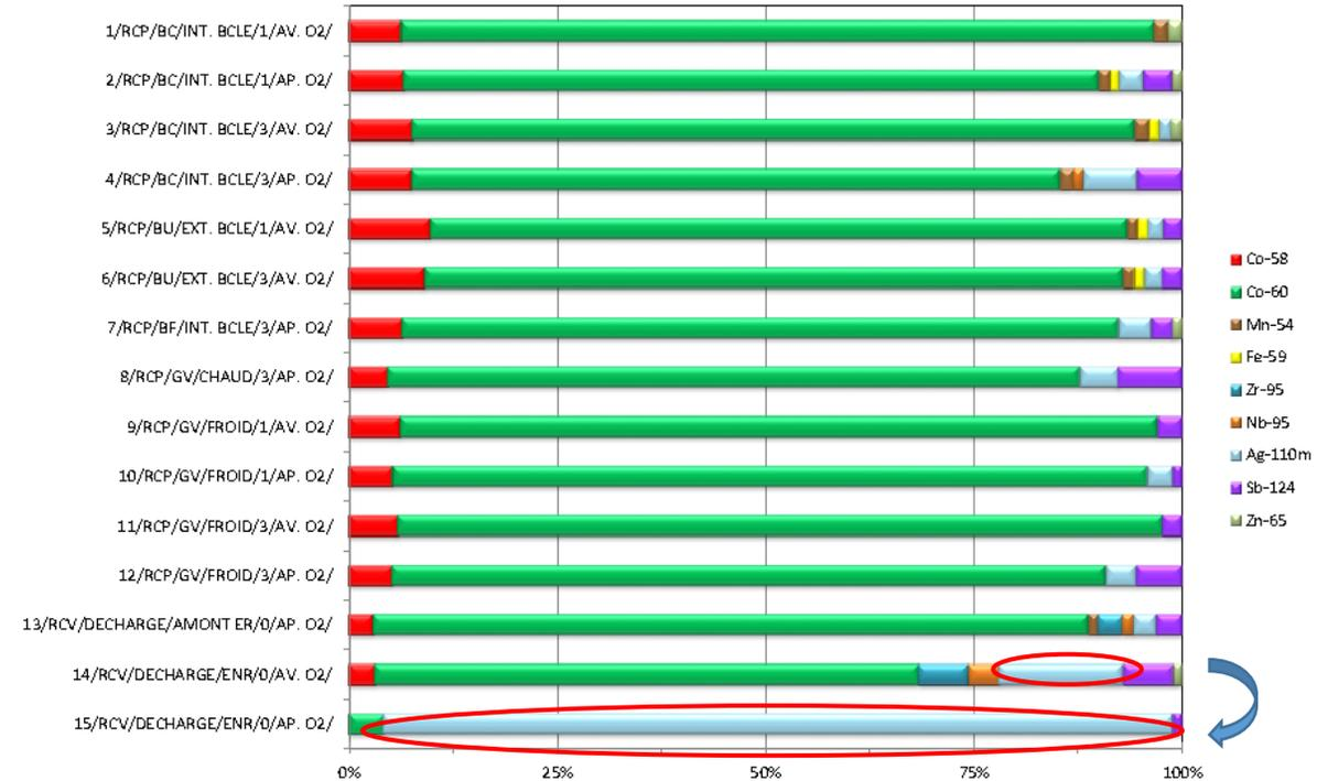
**A radionuclide that tends to deposit during forced oxygenation and mostly in the « cold parts » of the reactor. Dose rates can be increased by several decades.**
