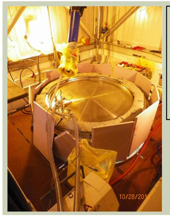
Borated Poly Shielding to Reduce Neutron Exposure
