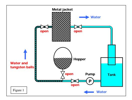
If only the water is allowed to drain in this condition, shields are completed. By using tungsten balls only in the isolated water path, tungsten balls themselves are not contaminated, and can be re-used, thus reducing the volume of waste materials.
