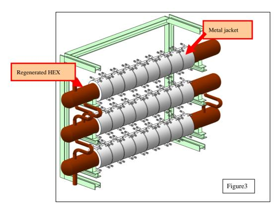
Tungsten balls are charged into this jacket one by one sequentially this way, and recovered also in similar way one by one sequentially.
