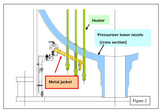
Metal jacket has holes to avoid the heater provided in the lower part of pressurizer, and provided at positions best to maintain work space and expect highest shielding effect.
