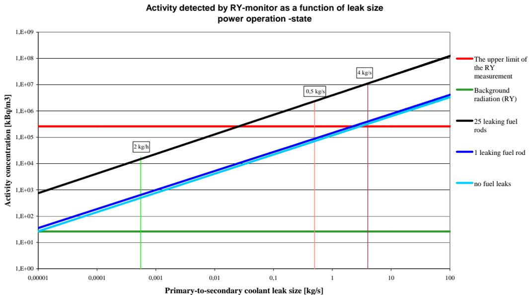
Figure 8. The relationship between leak size and activity detected by RY-monitor, power operation.
