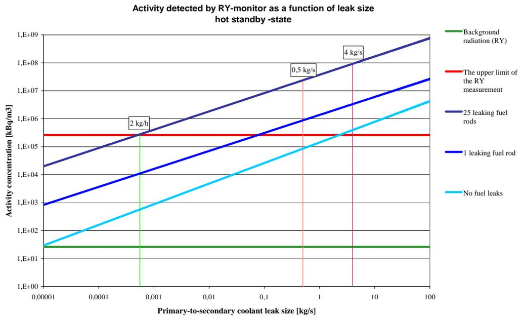
**Figure 10.** The relationship between leak size and activity detected by RY-monitor, hot standby
