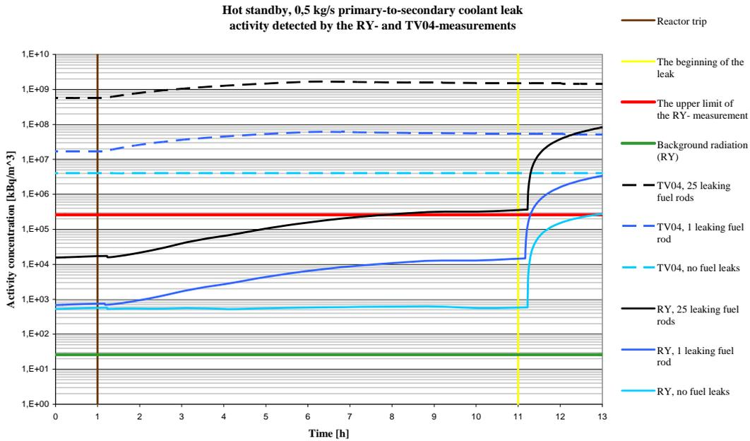
**Figure 5.** 0,5 kg/s p-to-s leakage in hot standby, RY- and TV04-monitors
