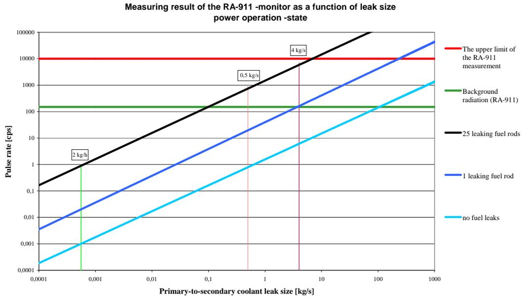
**Figure 9.** The relationship between leak size and measurement of the RA-911-monitor, power operation. Figures 10-11 are graphs of hot standby -cases:
