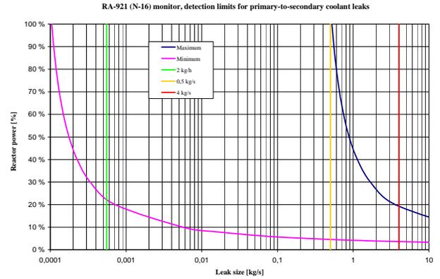
**Figure 1.** N-16 monitor's detection limits for the primary-to-secondary leaks
