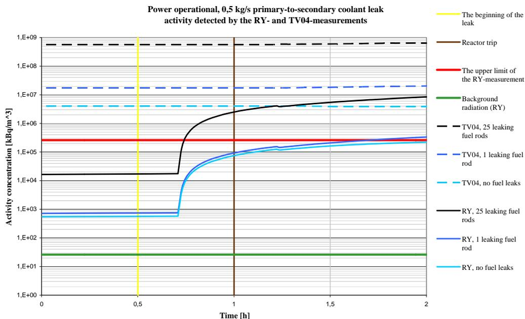
**Figure 4.** 0,5 kg/s p-to-s leakage in power operation, RY- and TV04-monitors
