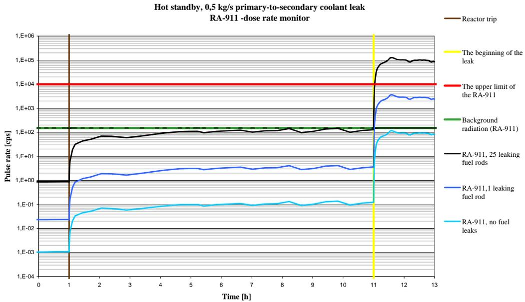
Figure 7. 0,5 kg/s p-to-s leakage in hot standby, RA-911-monitors
