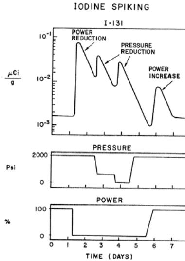
**Figure 2.** Schematic representation of iodine spiking [2].
