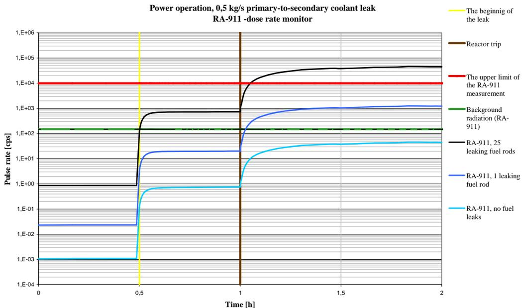
**Figure 6.** 0,5 kg/s p-to-s leakage in power operation, RA-911-monitors
