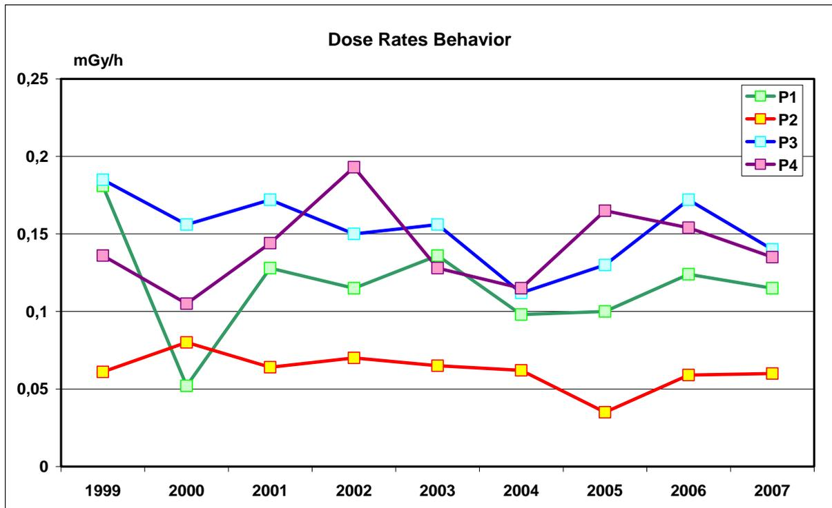
Fig. 6 – Dose rates measured directly on the main circulating loop insulation (insulation thickness, approx. 160 mm) at measuring points P1, P2, P3, and P4, 6<sup>th</sup> loop, Unit 4, Dukovany NPP, at about 50 hrs after unit shutdown
