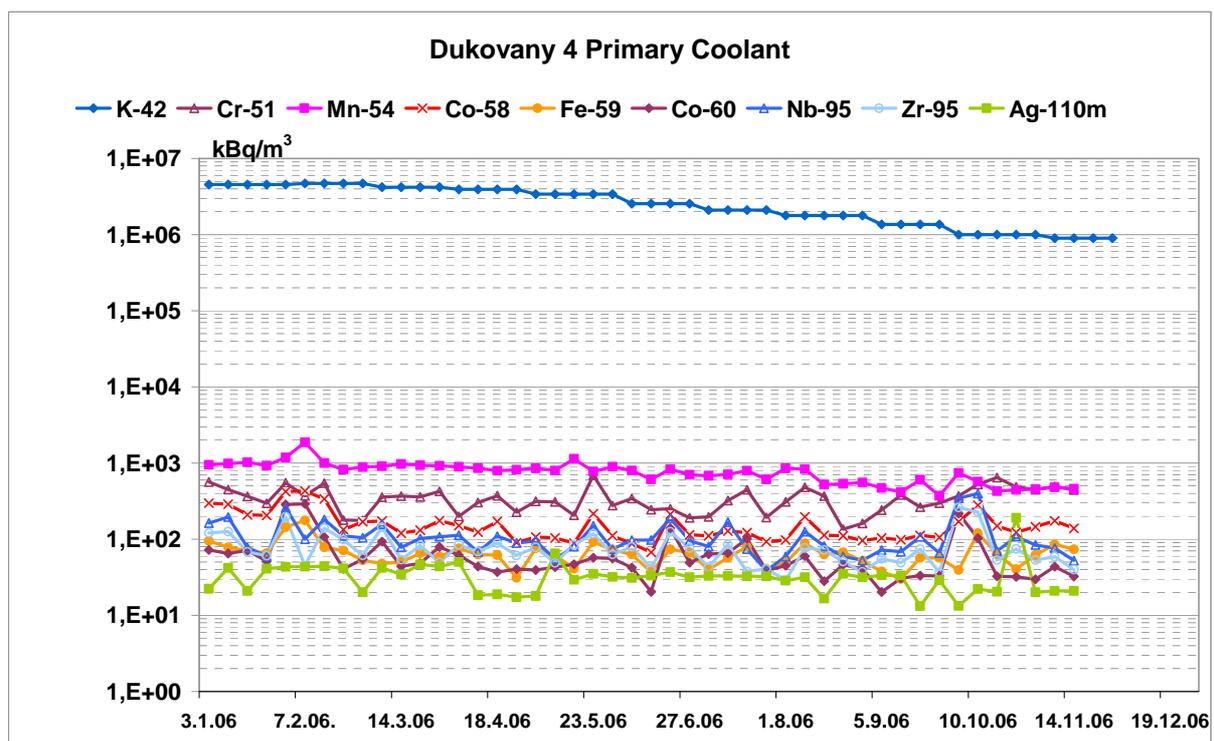
Fig. 1 – Volume activities of radionuclides in coolant of the Dukovany NPP primary circuit, Unit 4, 2006
