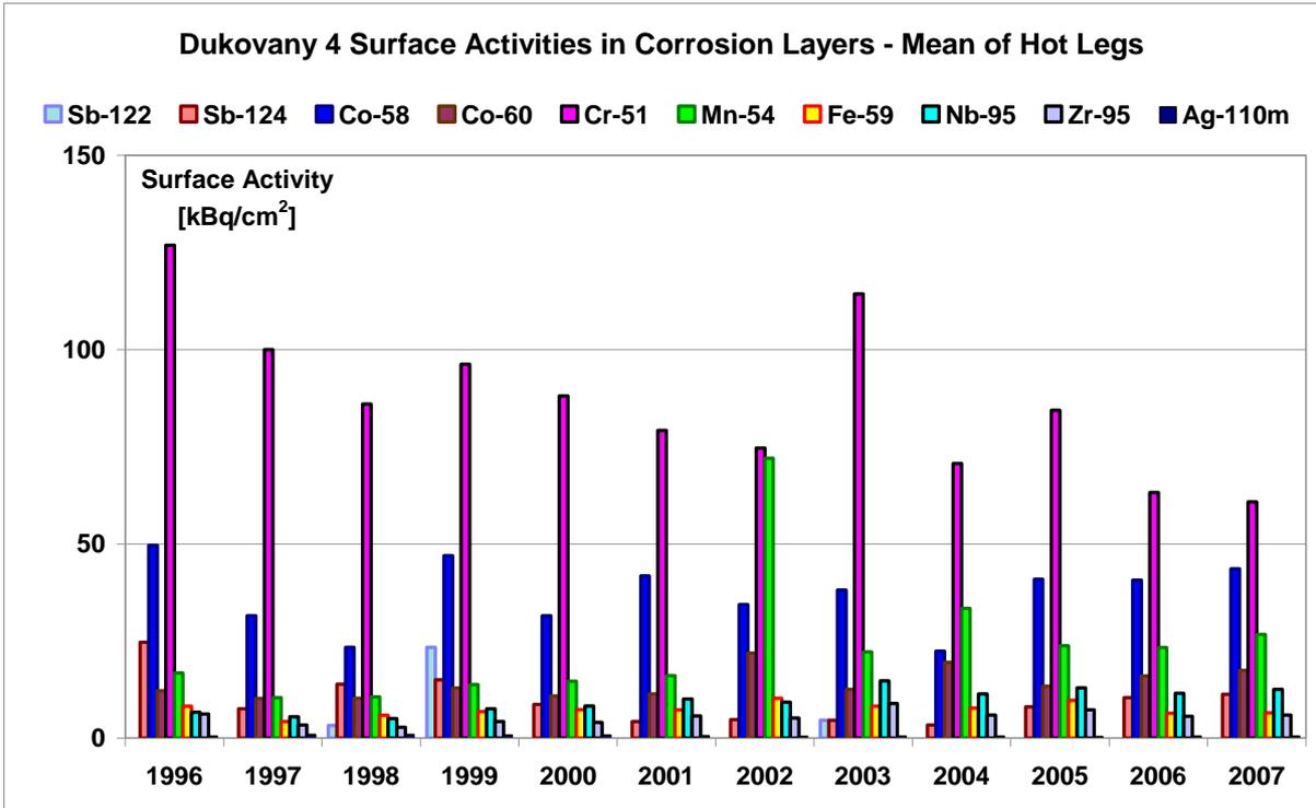
Fig. 2 – Surface activities of essential radionuclides on primary circuit surfaces of the Dukovany NPP, hot legs of Unit 4, 1996 – 2007
