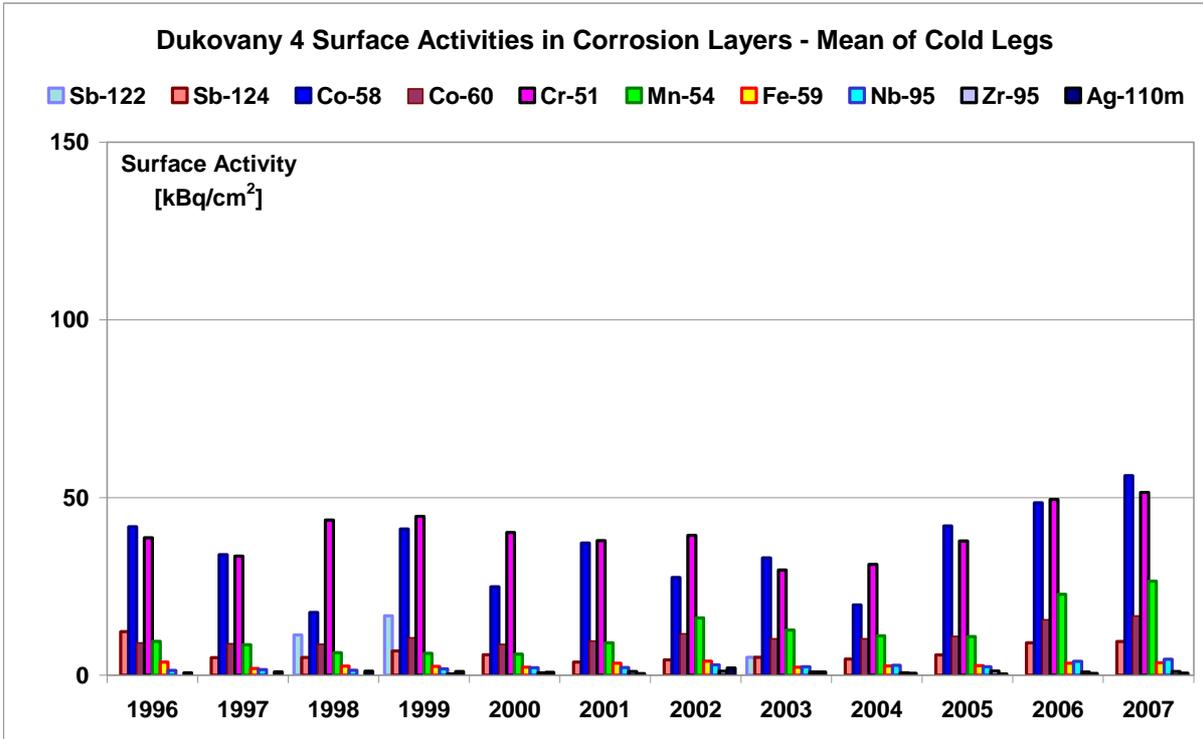
Fig. 3 – Surface activities of essential radionuclides on primary circuit surfaces of the Dukovany NPP, cold legs of Unit 4, 1996 – 2007
