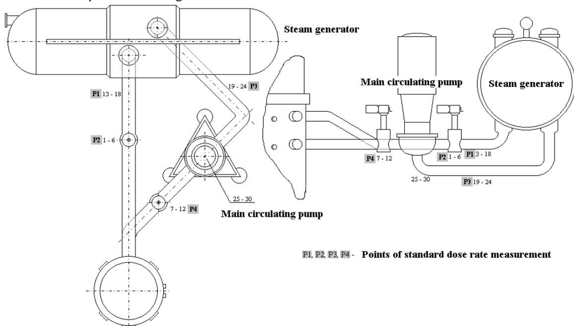
Fig. 5 – Dose rate measuring points according to the Dukovany NPP monitoring program
