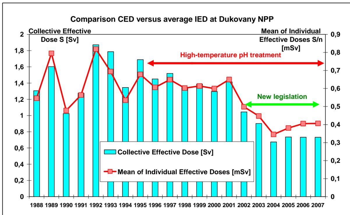
Fig. 8 – Collective effective dose and the mean of individual effective doses at four units of the Dukovany NPP, for IED > 0.05 mSv, from 1988 to 2007
