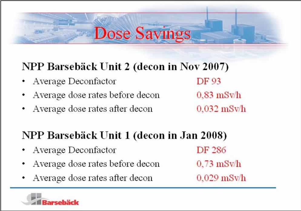
Figure 9: Overall DF results and dose rate reduction at NPP Barsebäck
