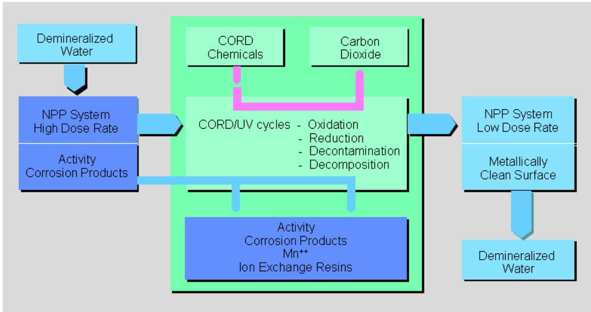
Figure 2: Principle of the HP/CORD UV Concept
