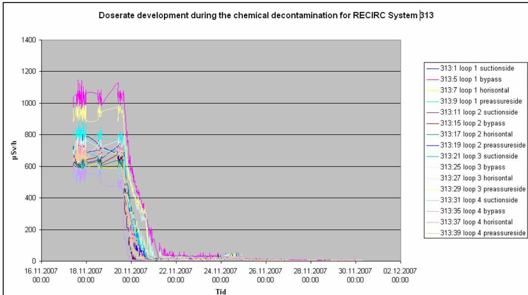
Figure 5: Doserate changes during the decontamination for the Recirculation System in Unit 2
