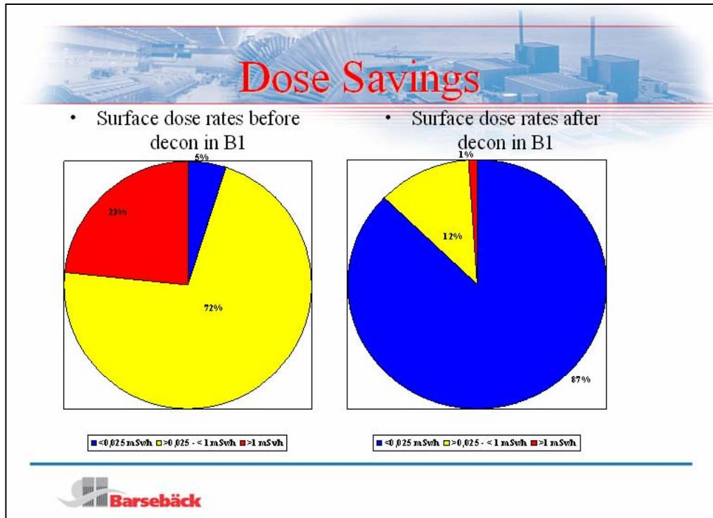
Figure 11: Changes in dose rates before and after the decontamination in Unit 1
