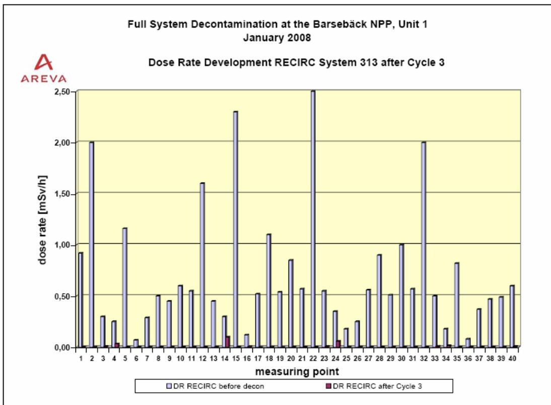
Figure 7: Dose rates of the Recirculation System in Unit 1 before and after the decontamination
