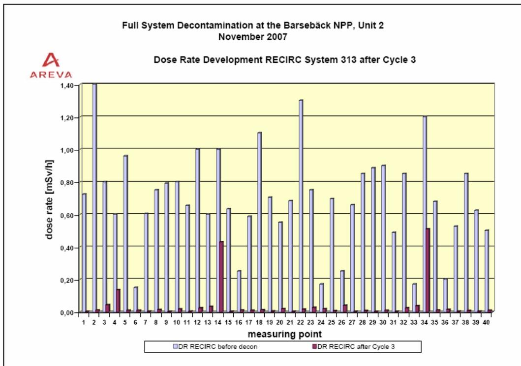
Figure 6: Dose rates of the Recirculation System in Unit 2 before and after the decontamination
