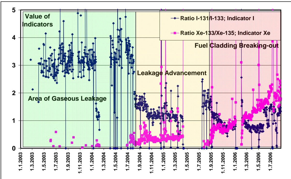
Fig. 4. Fuel cladding leakage indicators at Temelin NPP Unit 2 between 2003 and 2006
