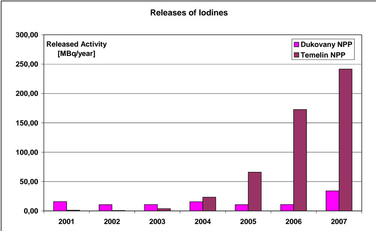
Fig. 7. Iodines in gaseous discharges
