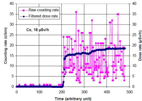
Fig. 5. Real time counting rate and filtered dose rate measured with a  $^{60}\text{Co}$  irradiator at 18  $\mu\text{Sv/h}$ .
