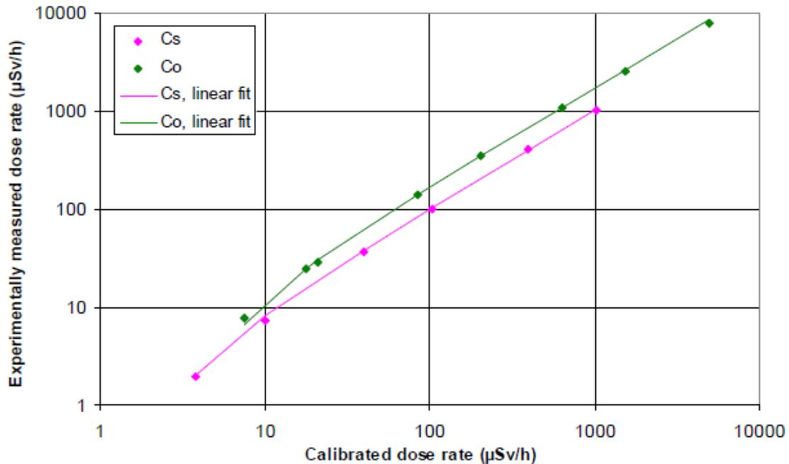
Figure 1 : Linearity of the dosimeter response with calibrated dose rate
