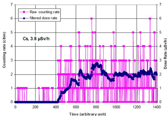
Fig. 4. Real time counting rate and filtered dose rate measured with a  $^{137}\text{Cs}$  irradiator at 3.8  $\mu\text{Sv/h}$ .
