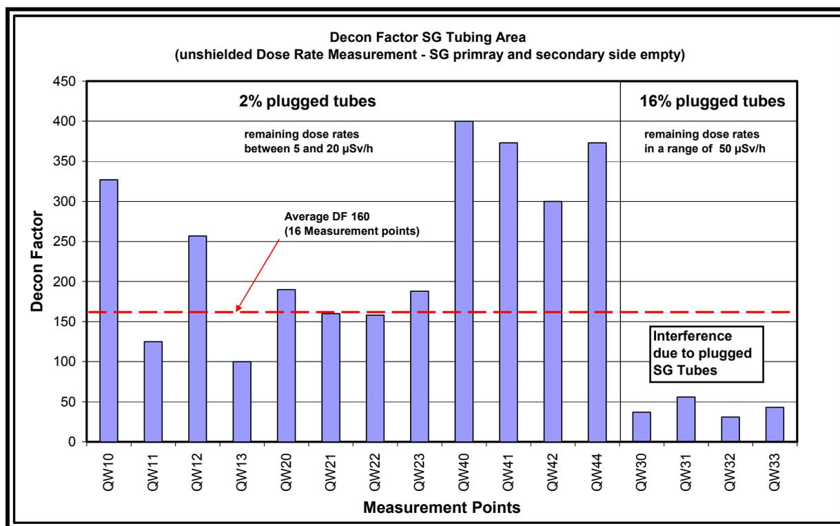
**Figure 1:** Steam generator decontamination factors for SGs 1 – 4
