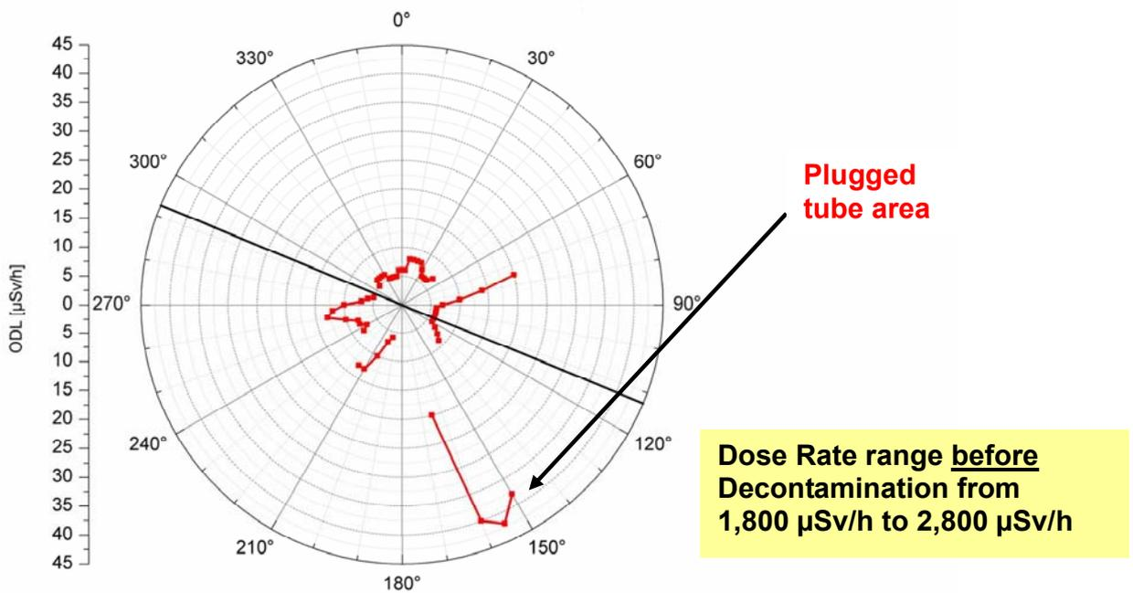
**Figure 2:** Contact dose rate of drained SG 4 after decontamination
