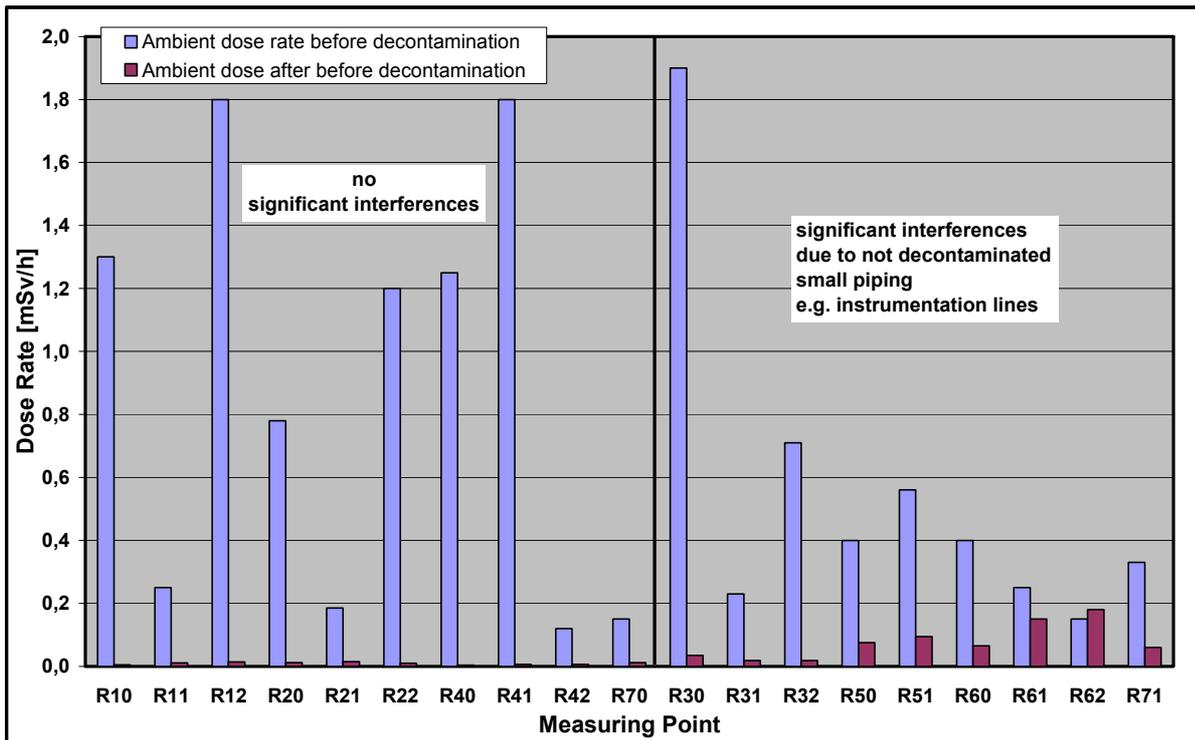
**Figure 4:** Ambient dose rates before and after decontamination (non-shielded measurements)
