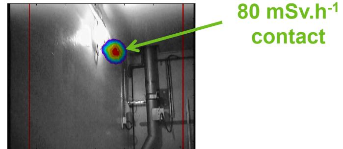
Detection of contaminated pipes
