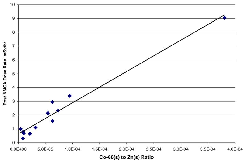
Figure 2: Measured post NMCA shut down dose rates vs. the reactor water Co-60(s) to Zn(s) ratio
