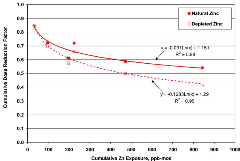
Figure 3: Cumulative dose reduction factor as a function of cumulative zinc exposure
