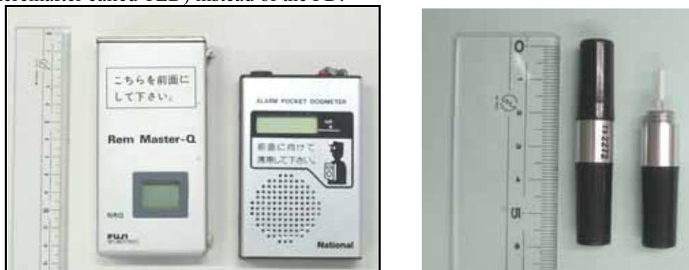
Fig. 2 Personal dosimeter with alarm function (left) and thermoluminescence dosimeter (right)
