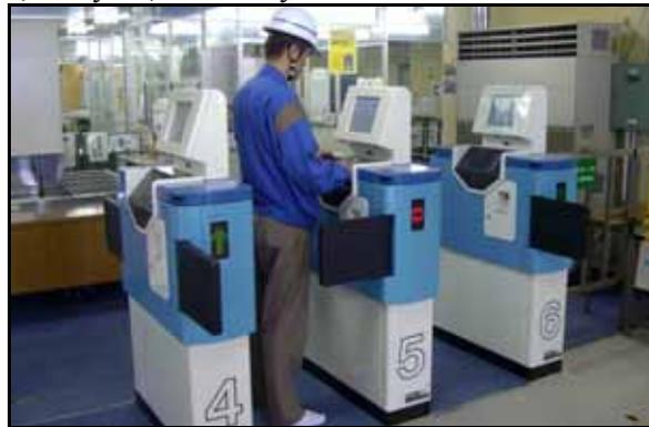
Fig. 5 Access control gates for electronic personal dosimeters for controlled areas
