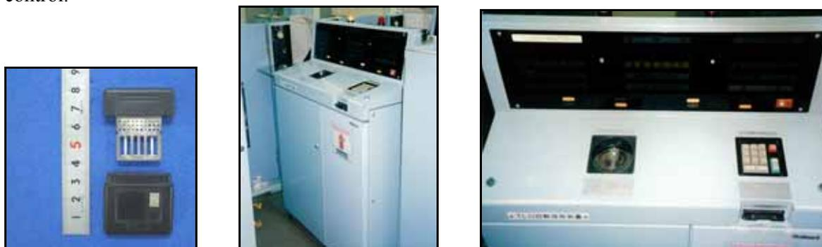
Fig. 3 Thermoluminescence dosimeter (left), access control gate (center), and operating section (right)
