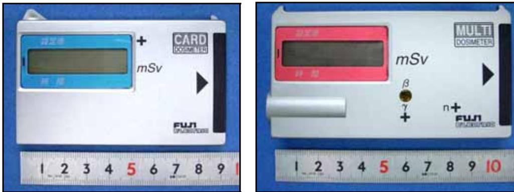
Fig. 4 Electronic personal dosimeter (left: for gamma rays, right: for gamma rays + beta rays + neutrons)
