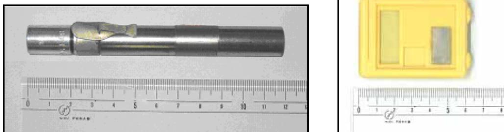
Fig. 1 Chamber-type pocket dosimeter (left) and film batch (right)
