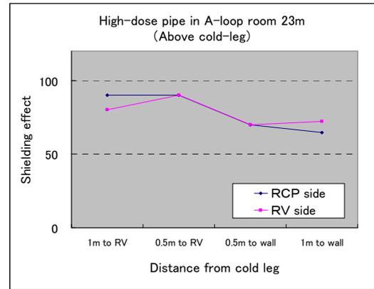
This temporary shielding is installed at places close to radiation sources. As a result, doses in large areas around the shielding will become low, effectively protecting workers who have to move around to perform their work.
