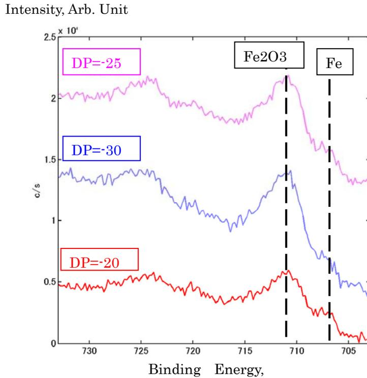
Figure 4 Fe<sub>2</sub>O<sub>3</sub> formed on the surface, showing effectiveness of dew point
