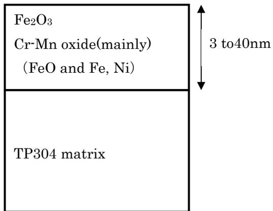
Figure 5 Multi-oxide layers in the pre-filming on TP304
