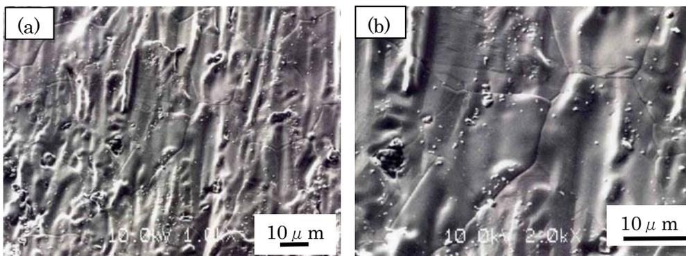
Figure 2 Morphology of the inner surface of the pre-filmed tube
