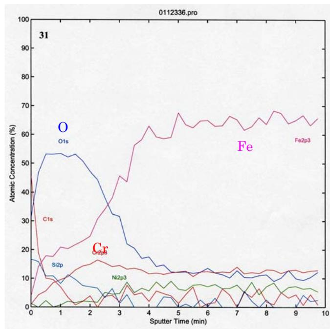
Figure 6 Depth profiles of the chemistries in pre-filming oxide
