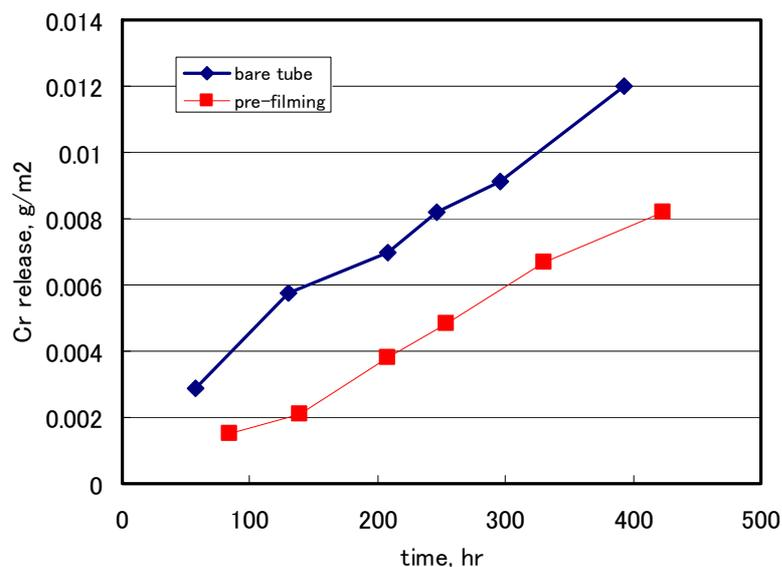
Figure 7 Relationship between test time and Cr release adding up in the refreshed type autoclave
