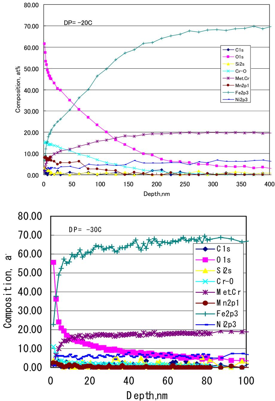
Figure 3 Depth profile of chemical analysis by XPS on the pre-filming surface
