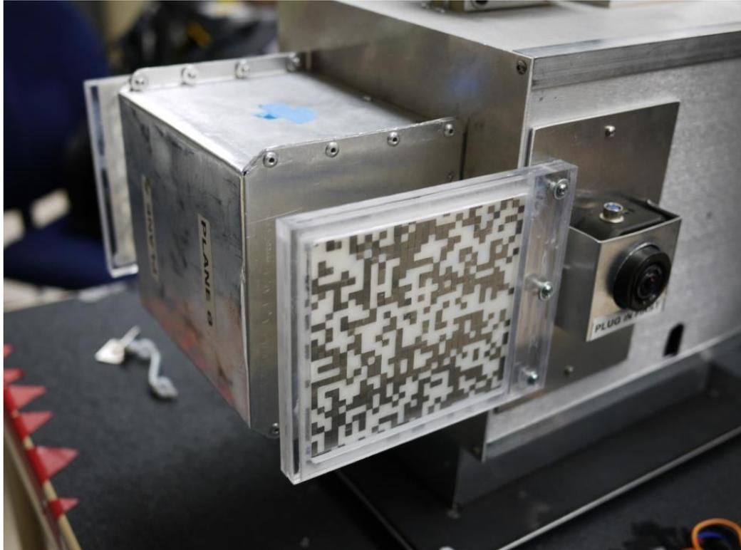
**Principle**: Recognize unique mask shadows from different incident gamma-ray angles
