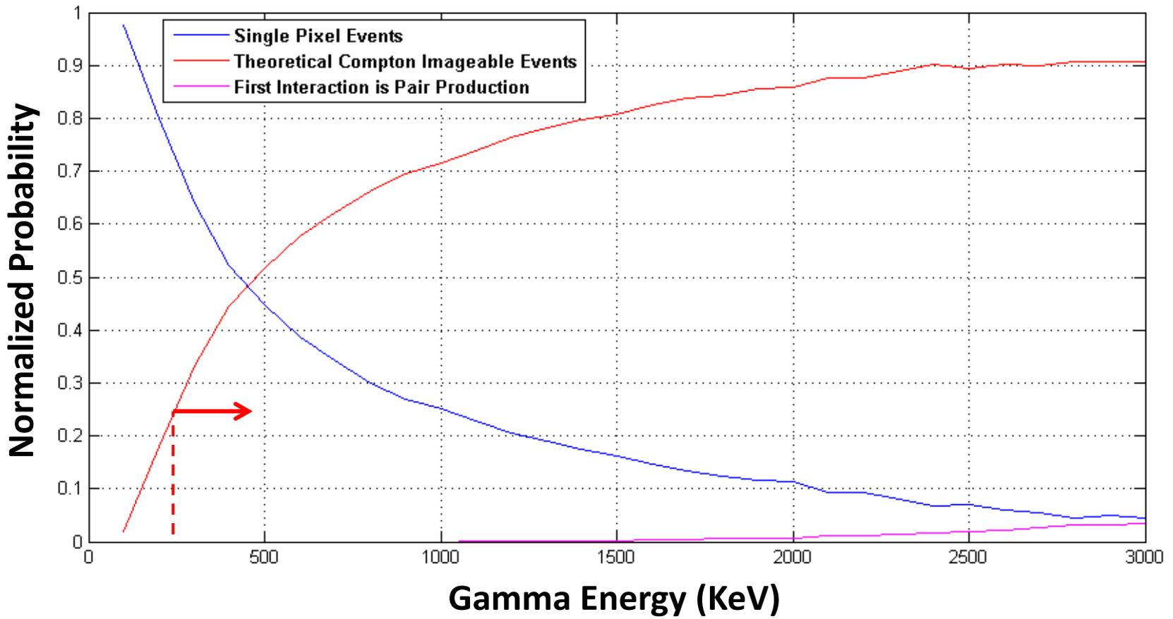
Polaris-H performs Compton imaging for  $\gamma$ -rays with  $E \geq 250$  keV
