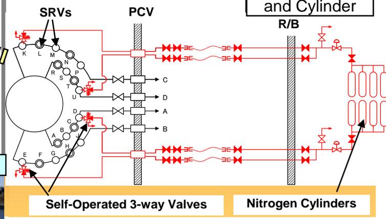
SRV Back-up Actuation Mechanisms
