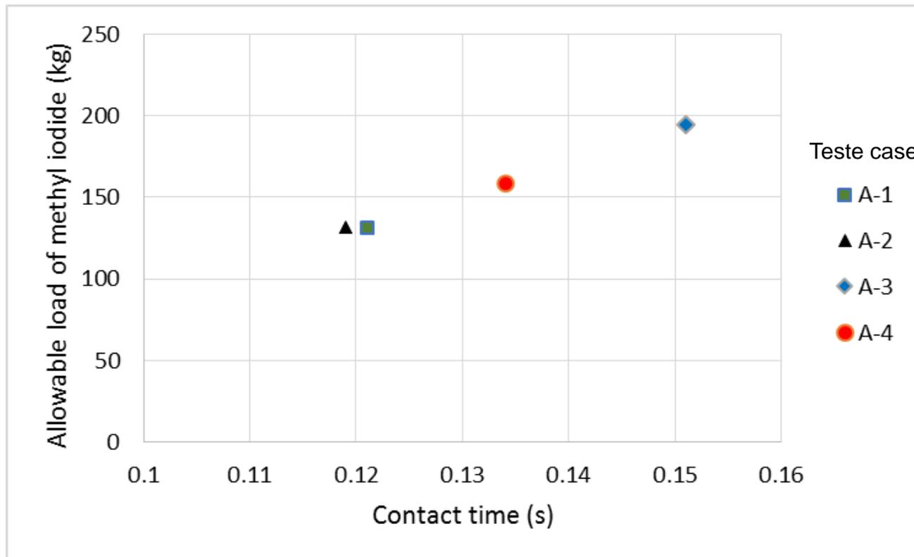
Relationship between contact time and allowable load of methyl iodide on two organic iodine filters for a plant.
