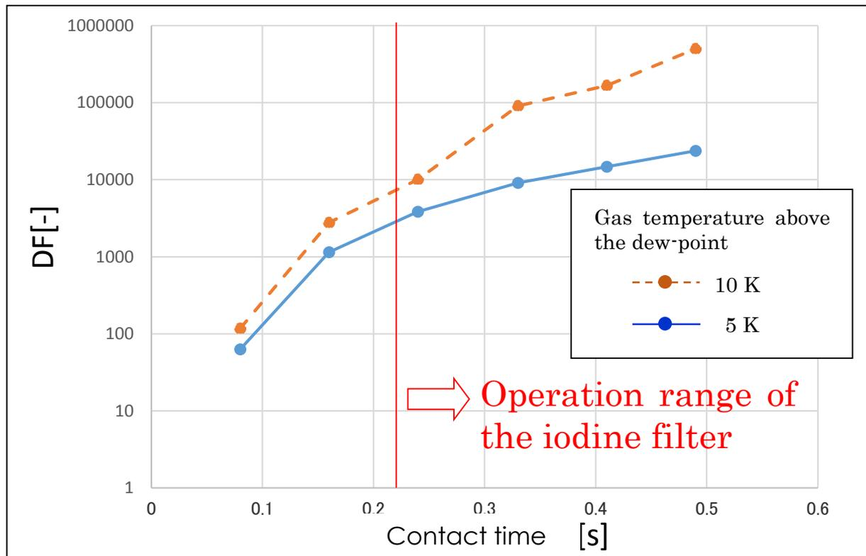
Methyl iodide decontamination factor of the iodine filter under steady state flow conditions
