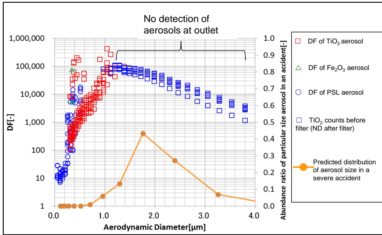
Aerosol decontamination factor (Maximum design flow condition)
