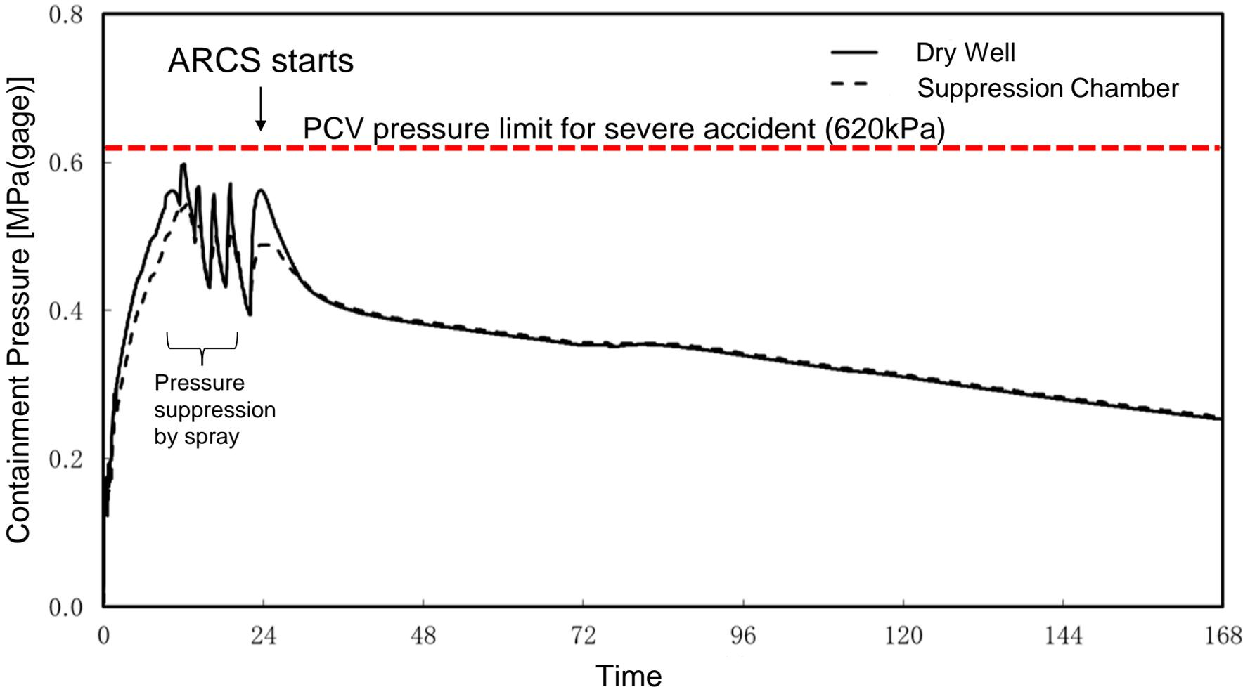
Containment pressure trend of Kashiwazaki Kariwa Unit 7 in a severe accident with large break LOCA, SBO, and loss of all ECCS
