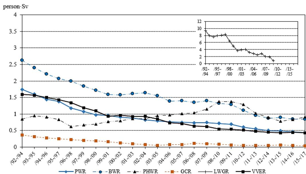
Note: PWR is pressurised water reactor; VVER is vodo-vodyanoy energy reactor; BWR is boiling water reactor; PHWR is pressurised heavy water reactor; GCR is gas-cooled reactor; LWGR is light water graphite reactor
