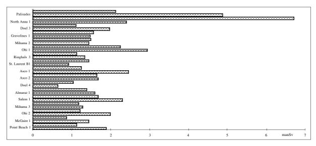
Figure 1. Evolution of steam generator replacement collective doses since 1990
