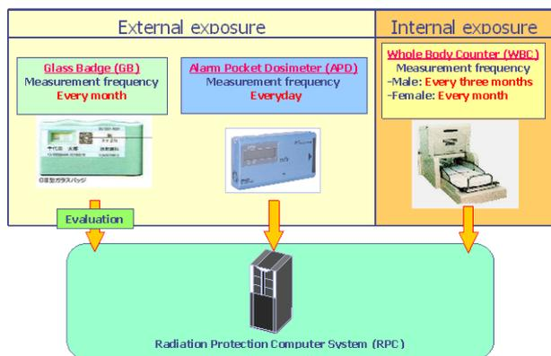
Fig.2 Measurement of exposure in Shika
