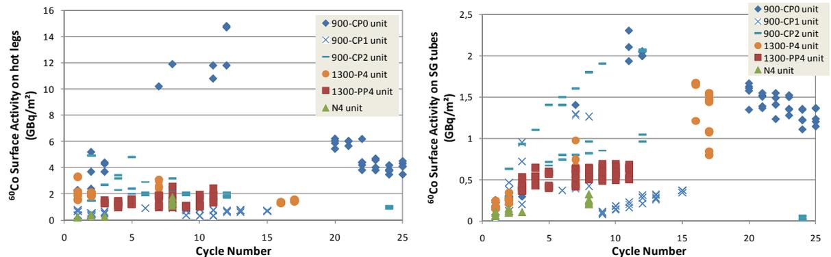
Figure 6: Evolution of  $^{60}\text{Co}$  deposited activities on hot legs (6a) and steam generator tubes (6b)
