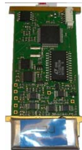
Figure 2 : Electronic board with the CZT
