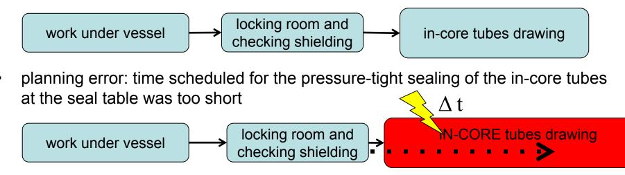
to fix this problem, the beginning of in-core tube withdrawing was brought forward without recognizing the conflict with the work in the reactor cavity room
