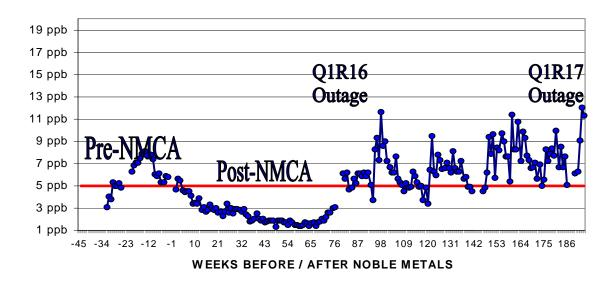
During cycle 17, DZO has been maintained in the 5-10 ppb range. Additionally, hydrogen cycling has been minimized. The soluble and insoluble Co-60 levels have stabilized and even begun to decrease, particularly in the case of the soluble form.
