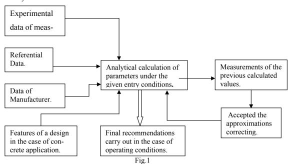
Calculation algorithm used the data of EDR measurements from the container loaded with a nominal SNF, the container design specific features, the container configuration for such usage, work performance procedure technique, and also tabulated and analytical formulas of calculating radiation protection. The subsequent comparison of the measured values of equivalent dose rate with precomputed dose rate has shown correctness of the calculation algorithm: the divergence did not exceed 3 per cent.
