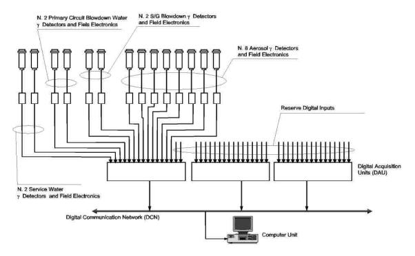
Figure 3 - Radiation MonitoringSystem - Connection of New Monitors to the new Computer System
