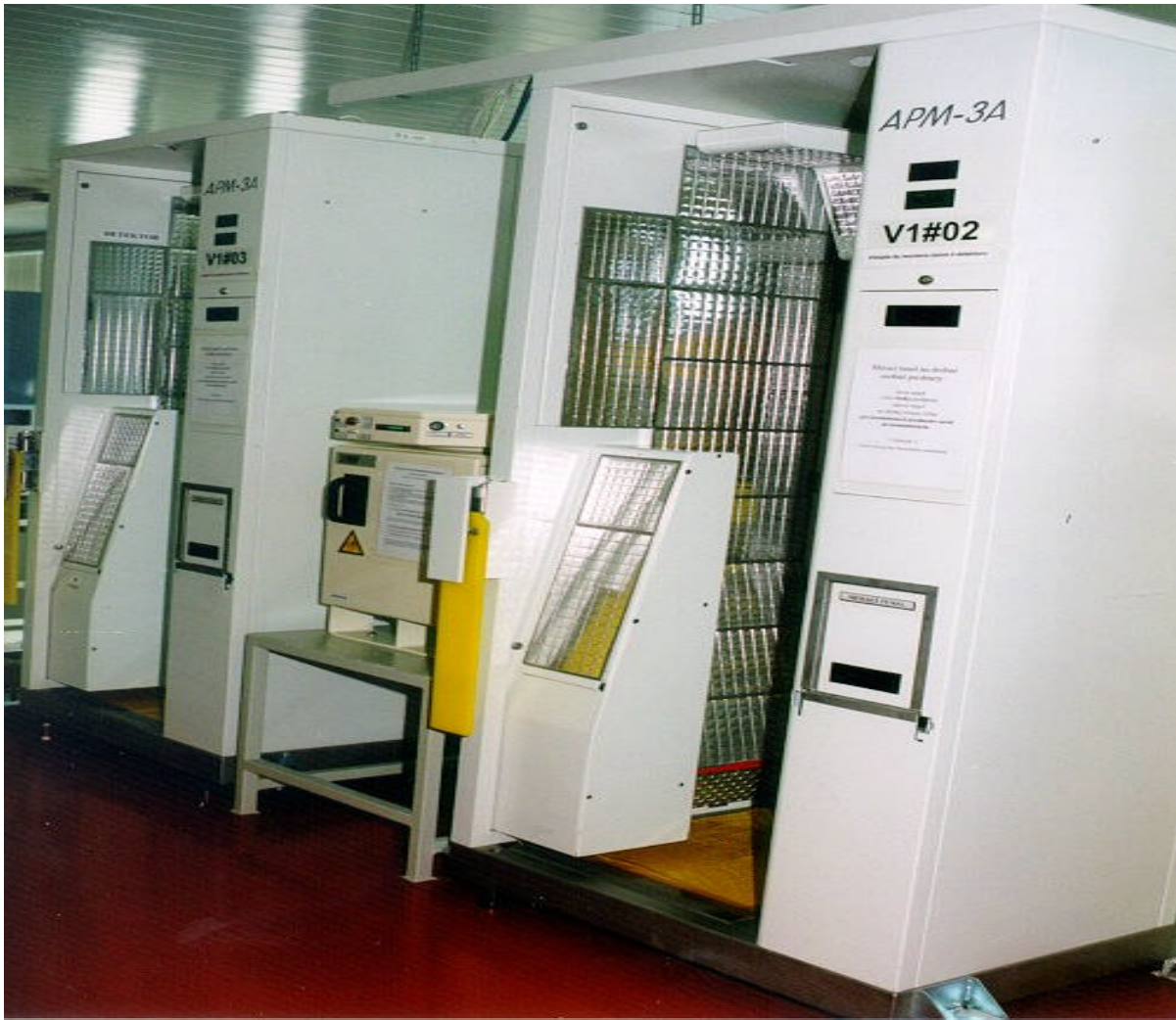
Fig. 1: CPO and APM-3A monitors
