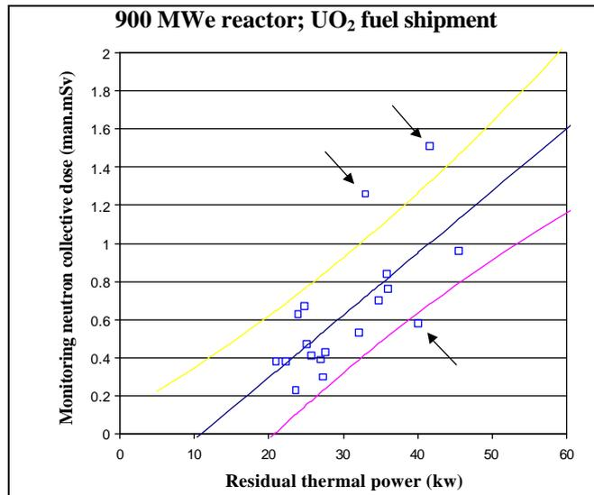
**Figure 2: Linear regression between monitoring neutron collective dose and residual thermal power (900 MWe reactor, UO<sub>2</sub> fuel shipment)**
