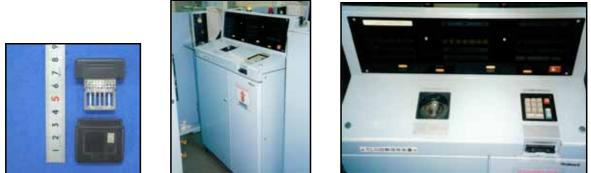
Fig. 3 Thermoluminescence dosemeter (left), access control gate (center), and operating section (right)
