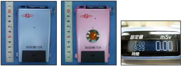
Fig. 6 Advanced E.P.D. (left: for gamma rays, right: for gamma rays + beta rays + neutrons) and dose display
