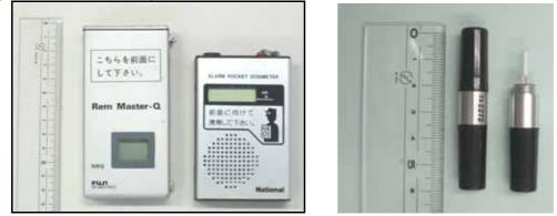
Fig. 2 Personal dosemeter with alarm function (left) and thermoluminescence dosemeter (right)
