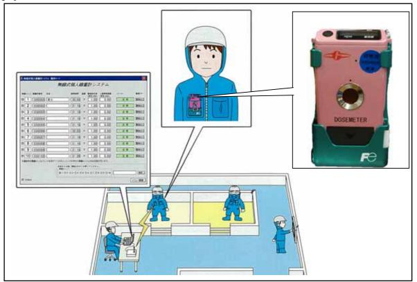
Fig. 7 Conceptual diagram of wireless monitoring system
