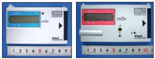
Fig. 4 Electronic personal dosemeter (left: for gamma rays, right: for gamma rays + beta rays + neutrons)
