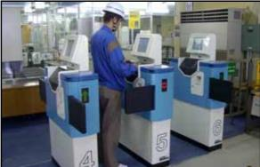
Fig. 5 Access control gates for electronic personal dosemeters for controlled areas
