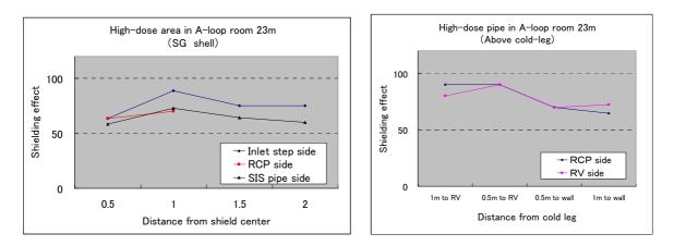
This temporary shielding is installed at places close to radiation sources. As a result, doses in large areas around the shielding will become low, effectively protecting workers who have to move around to perform their work.
