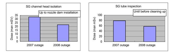
Dose reduction in SG channel head work - 31.7% Dose reduction in SG tube inspection - 26.9%
