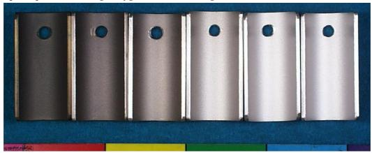
Figure 1 The inner surface pre-filmed under the laboratory conditions showing the effectiveness of dew point during heat treatment
