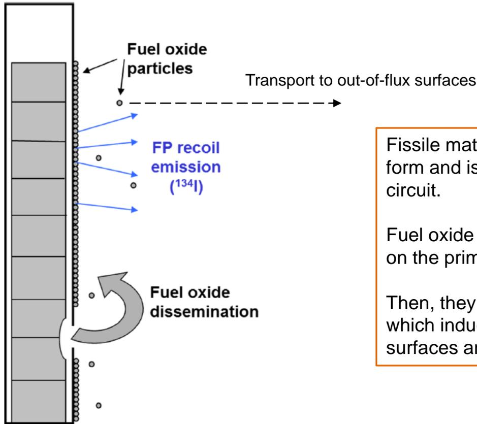
Fissile material disseminates in particulate form and is mainly insoluble in the primary circuit.
