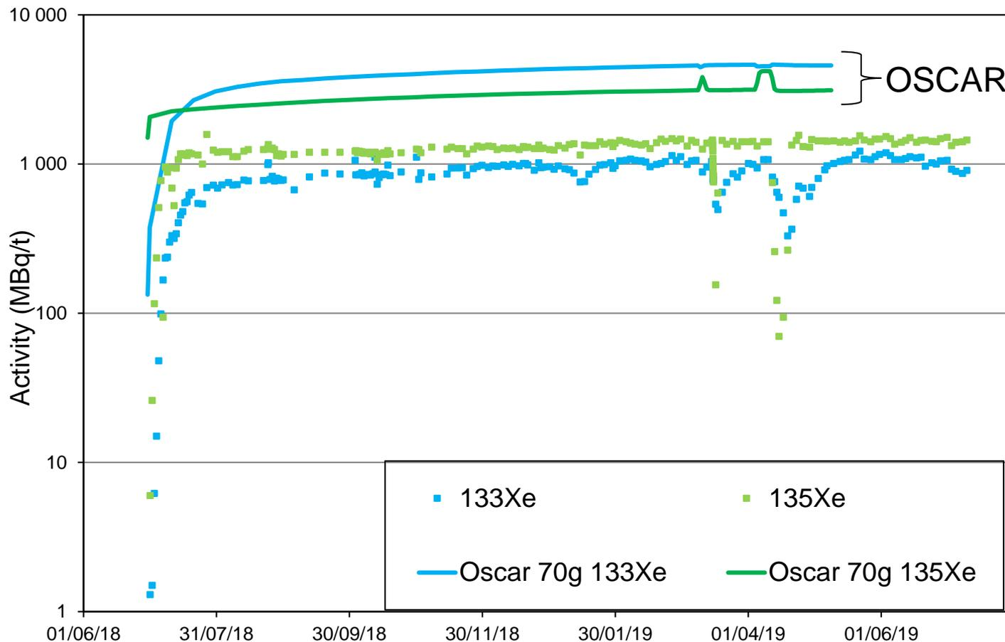
The OSCAR calculation shows that without any defective fuel rod, the activity in Xe-133 and Xe-135 remains high due to the residual contamination (previous cycle « ii »)
